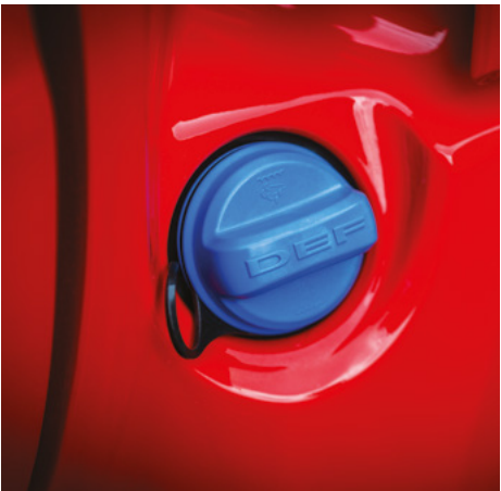
The diesel exhaust fluid (DEF) tank fill point is located near the passenger side door to help avoid mixing the wrong fluids and allows the tank to be filled without opening the hood
