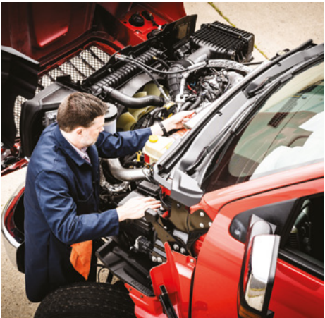
The Forward-tilting hood provides easy access to the engine and routine service points
