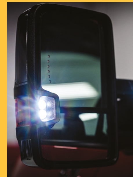
The folding side mirrors can include LED turn indicators plus rear-facing LED lights to illuminate cargo and equipment.
